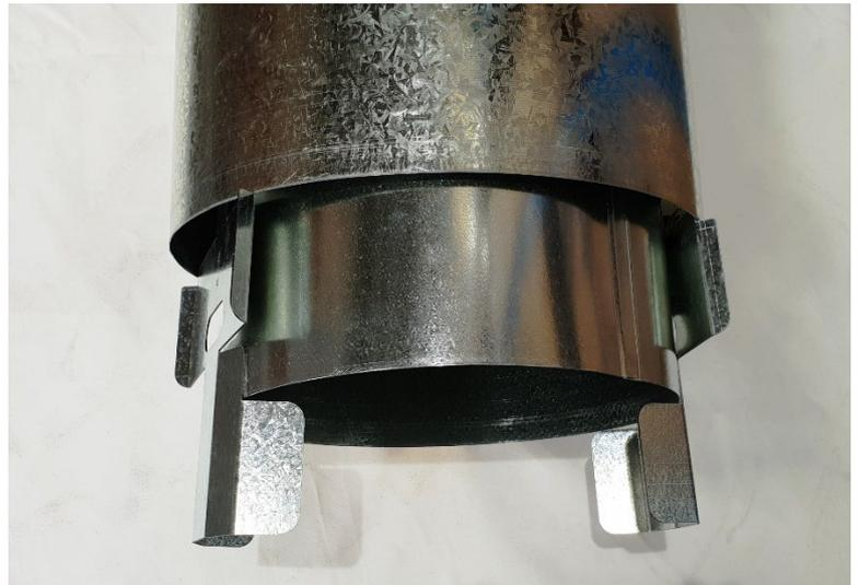
The 10" slides through the top of the Zero Clearance Box and sits above the heater resting on the brackets. The 10" MUST be sealed with a flexible sealant around the top of the Zero Clearance box to stop heater air coming into the chimney chase cavity.
