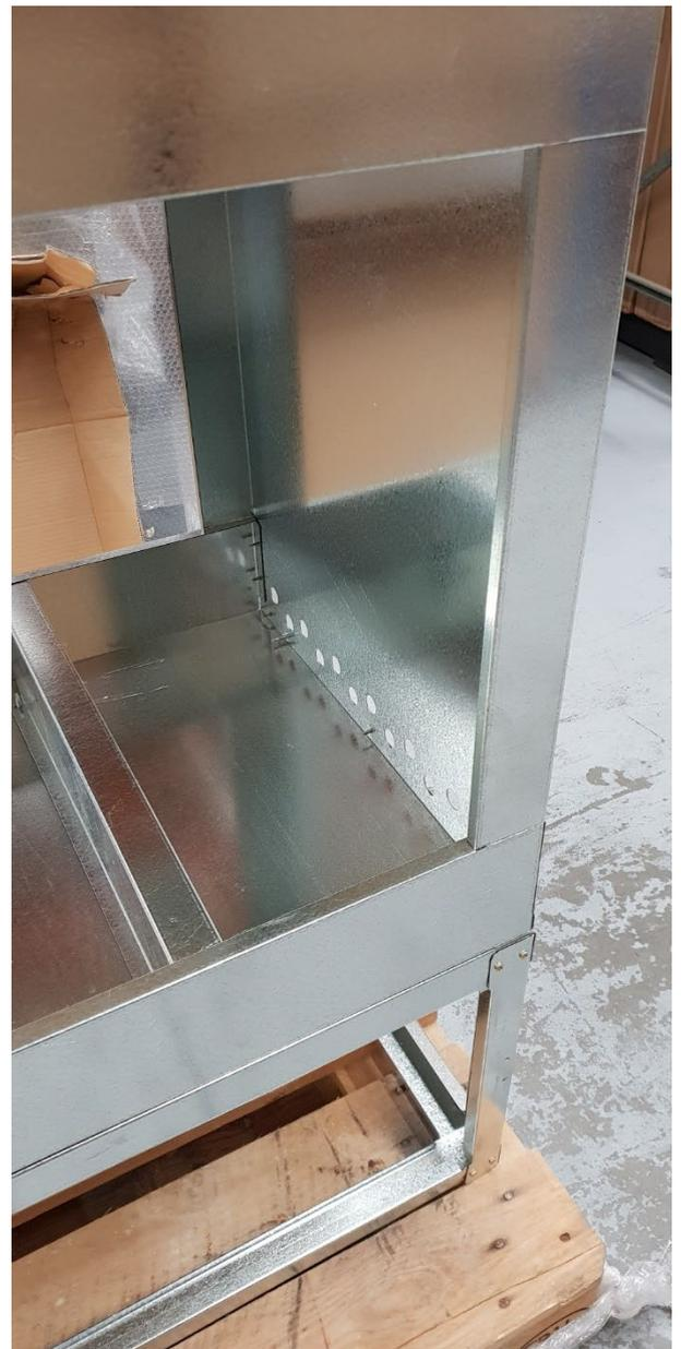
NOTE: When screwing 2 panels together through the existing holes , the screw should go through the larger hole first, then through the smaller hole, and cutting the thread in the smaller hole. In some holes may screw from the inside, some from the outside.
