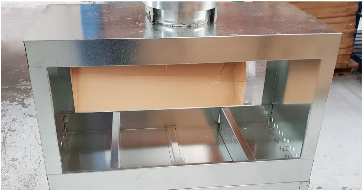
The top panel fits on, with the folds on the outside of all the other panels. Alternatively it could be fitted on the inside of the side panels, so the holes are the same size.
