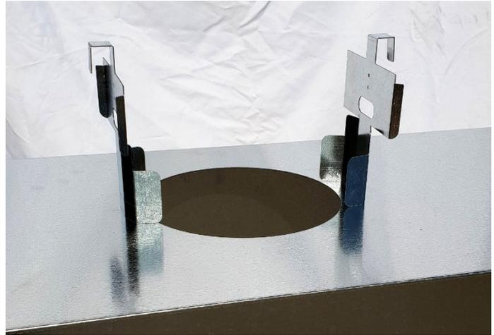
The brackets are fixed to the 10" inner casing and then the upper folded U shaped hook is fixed to the 12" outer casing. These can be fixed with self tapping screws or rivets.
