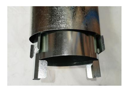
The 10" slides through the top of the Zero Clearance Box and sits above the heater resting on the brackets. The 10" MUST be sealed with a flexible heat resistant fire cement sealant around the top of the Zero Clearance box to stop heater air coming into the chimney chase cavity.
