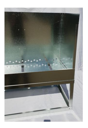
NOTE: When screwing 2 panels together through the existing holes, the screw should go though the larger hole first, then through the smaller hole, and cutting the thread in the smaller hole. Ie some holes may screw from the inside, some from the outside.
