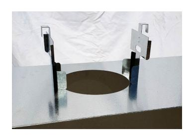
The brackets are fixed to the 10" inner casing and then the upper folded U-shaped hook is fixed to the 12" outer casing. These can be fixed with selftapping screws or rivets.
